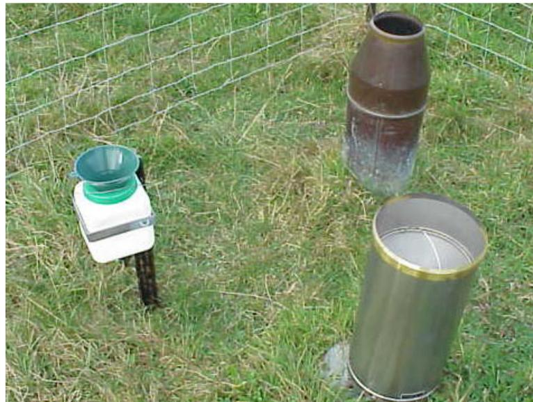
**Figure 2.3:** Mangemangeroa (Howick) rainfall station (Map 260 R11, 8250E 7220N). The rainfall sampler for  $^{210}\text{Pb}$  deposition measurements (left) is serviced at monthly intervals. An automatic tipping bucket (front right) rain gauge provides rainfall intensity-duration data.
